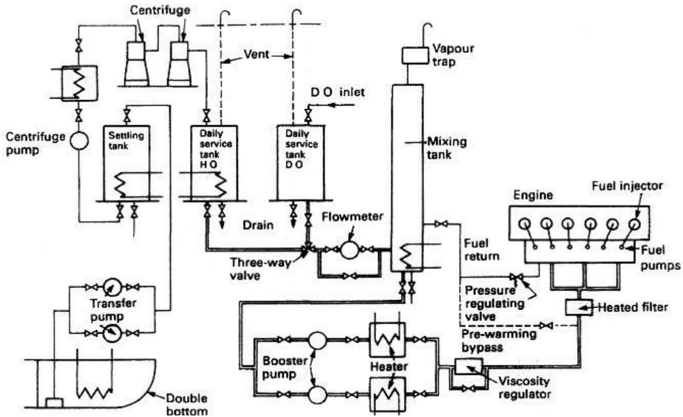
Fig: Fuel oil system for cargo ships
