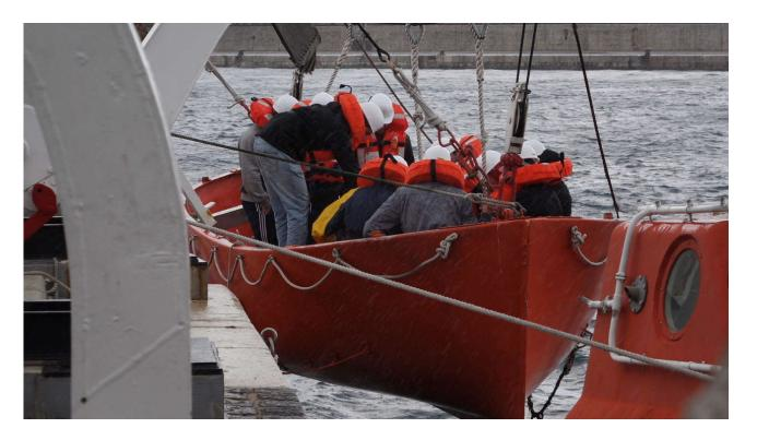
4. **Fast rescue boat** is moored in the water area of the Practicum. It is equipped with an outboard engine Suzuki DF90 ATL 66.6 kW and has all the equipment in accordance with the SOLAS convention. The boat has the following technical characteristics:
