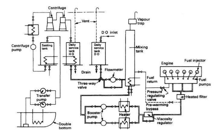
Fig: Fuel oil system for cargo ships
