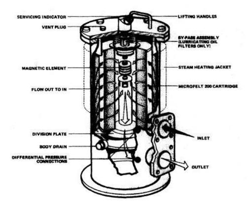
A felt-type fine filter is shown in Figure
