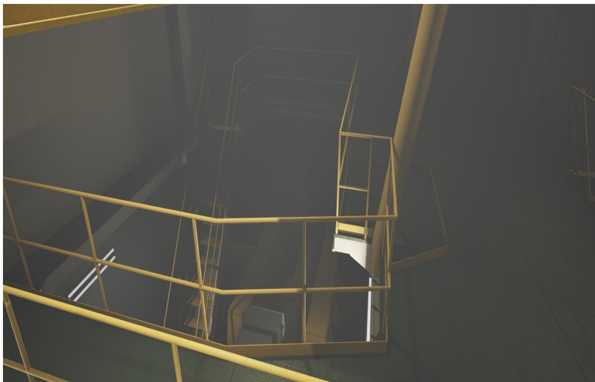
Figure 59 – CFD imported smoke data of fire of oily rags left in a bucket scenario to the VR engine room
