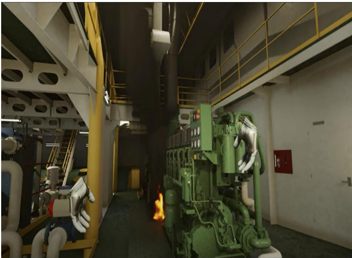
Figure 58 – CFD imported smoke data of fire of the main engine fuel line scenario to the VR engine room.
