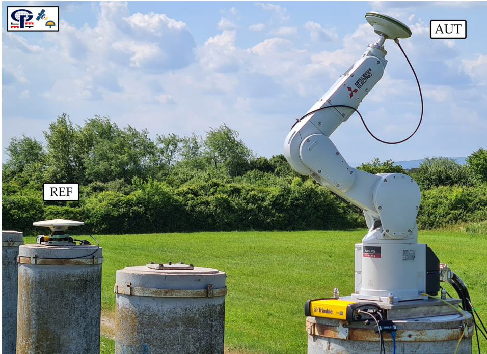
Figure 1. On-site set-up of the LMMT antenna calibration system [7]. The industrial robot Mitsubishi MELFA RV-4FLM-Q with the installed antenna-under-test (AUT) Leica Geosystems AX1202 GG and the reference (REF) antenna Trimble Zephyr 2 Geodetic. Baseline length is approx. 5 m. Both antennas are connected to Trimble NetR5 GNSS receivers.
